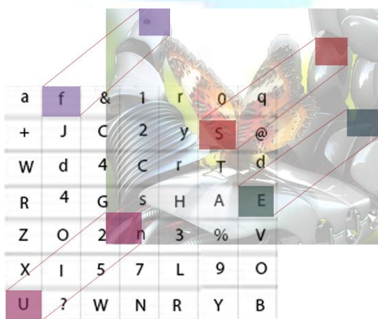
Fig.5. Selecting the position in the PatternSquare by touching the particular portion of the image.
